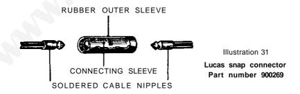
One snap connector is used in the rear lamp wire and another is used in the wire connecting the regulator unit to the output side of the ammeter in the head lamp.
