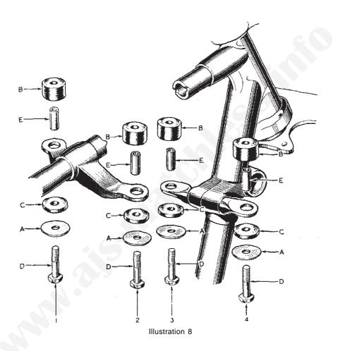
Showing details and order of assembly, of the fuel tank fixing bolts and components
