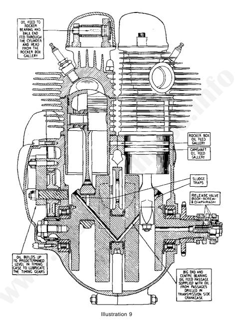
Cross section of engine showing oil galleries, oil passages, and release valve.
