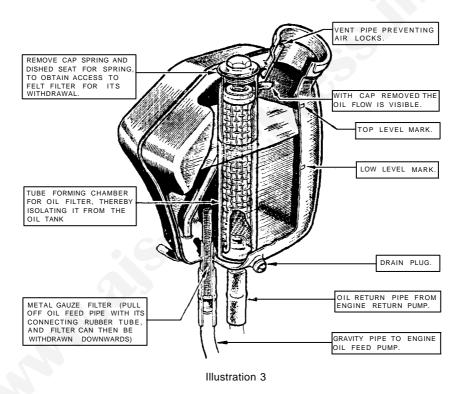
Showing the oil tank with the felt filter in its cylindrical housing and the metal strainer mounted on the entry end of the feed pipe union. Also shows the direction of flow of oil from tank to engine and return flow from engine to tank via the small spout, located so that it can be inspected by removing the tank filler cap. An air vent pipe is provided to ensure freedom from air-locks.
